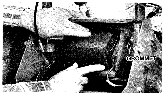
Photo 5-53: Installing the battery.
